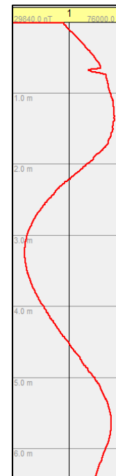
Figure 12. Data trace of 2.5m ferrous anomaly.
