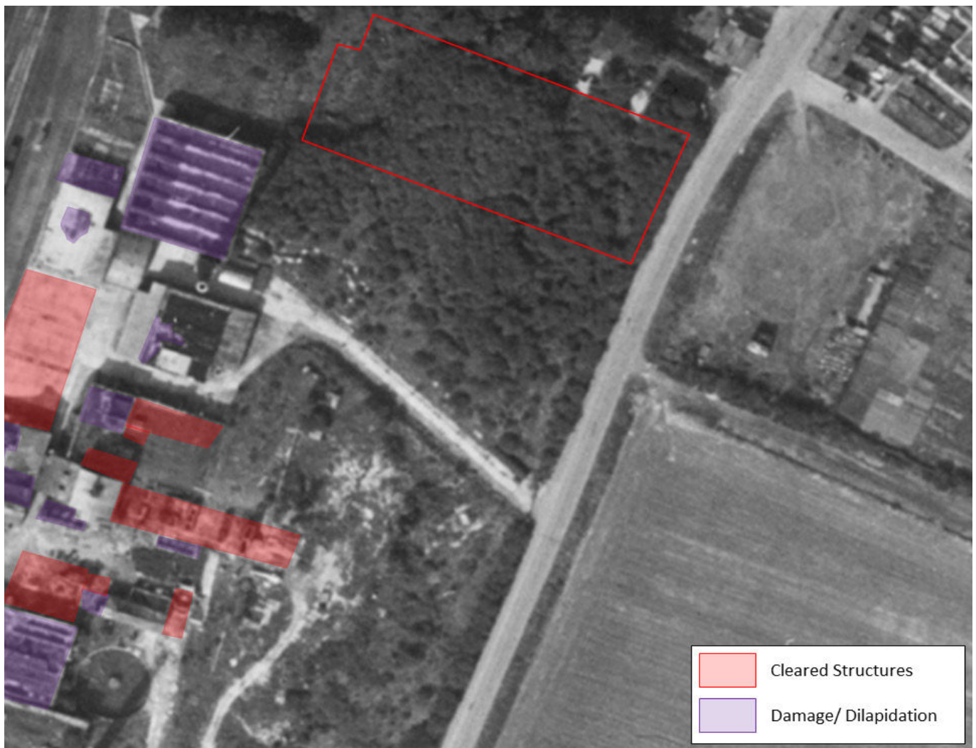
Aerial photography taken in 1948 of the development site in Arlesey, Bedfordshire – which needed to be investigated for UXO contamination. The red overlays highlight previously cleared structures and the purple overlays highlight previous structural damage close to the site boundary area – highlighted by the red keyline.
