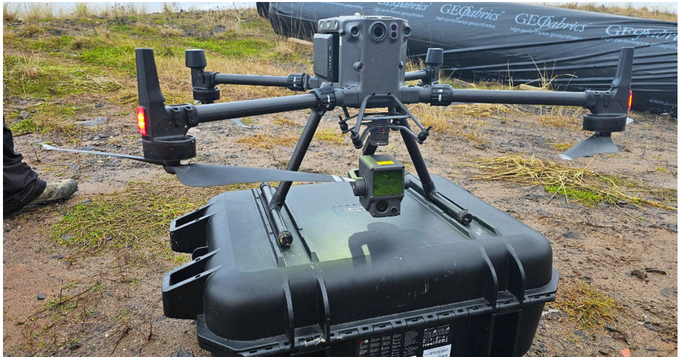
Aerial / Drone fitted with L1 camera payload.
