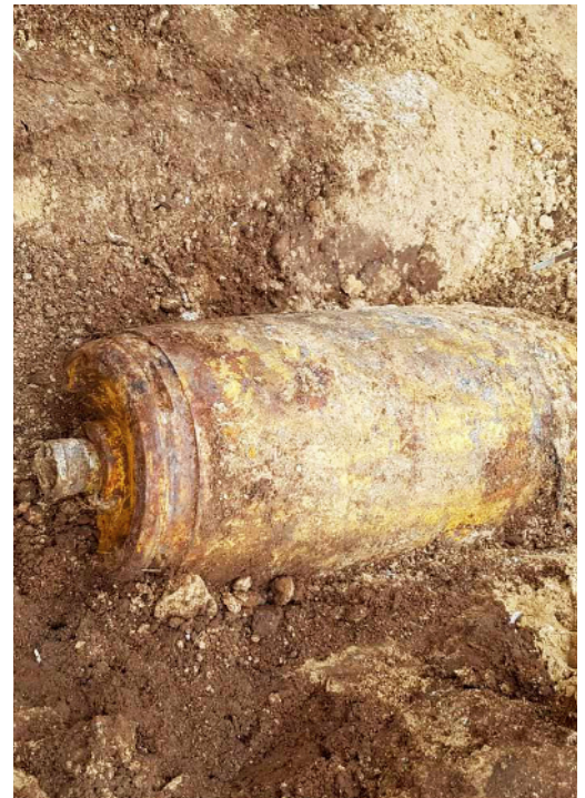
Close-up image of a British 500lb HE unexploded bomb found during Target Investigation at a site in Thetford, Norfolk.
